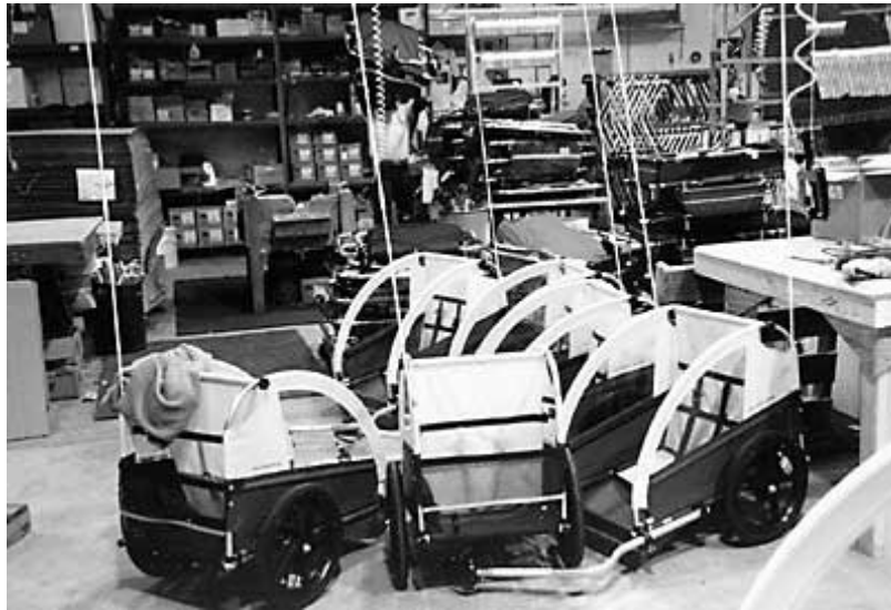
Burley trailers sit in the assembly area near the end of the production process. Visible on the trailer to the far right is the unique and versatile single arm hitch that allowed the Burley trailer to attach to almost any bicycle and helped, along with its small wheels and low center of gravity, to make the trailer Burley's most famous product. The hitch could also be mounted with a third wheel, turning the trailer into a stroller.
