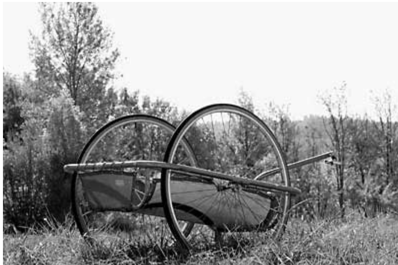
Burley's first trailer was fashioned from a used swing set. The prototype pictured here became the basis for Burley's signature trailer, and the basics of the design remain influential in the company's "Flatbed" and "Nomad" trailers to this day.
